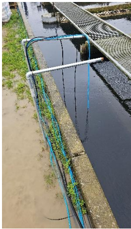
OxyGuard DO, CO 2 and pH sensors.
